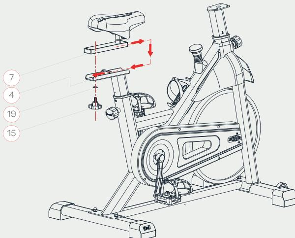
Install the saddle adjustment frame (7) on the saddle frame (4), and secure it with a flat washer (19) and an adjustment nut (15). Remember to loosen the adjusting nut (15) to move the seat adjustment frame (7) forward and backward as needed. Do not forget to tighten the adjusting nut (15) before use.
