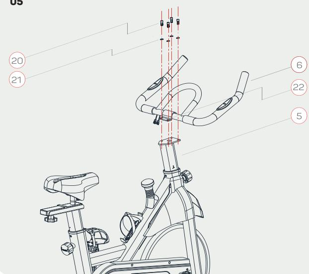
The next step is to attach the handle frame (6) to the handle post (5) using flat washers (17), spring washers (21) and socket head cap screws (20). Secure with an Allen key (27).
